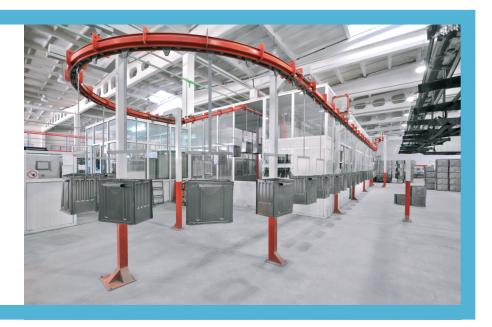
The cooking chambers are coated fully automatically with glass ceramic powder by a painting robot and then cured in an oven at temperatures of 850°.
