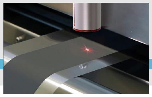
OptiSense technology checks the coil, a long, narrow electrode strip
