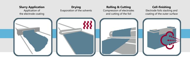
the cathode material (lithium compound) on aluminum foil. The short measuring time of the OptiSense technology is ideally suited for the contactless inline characterization of the calendering process in lithium-ion battery production. For this purpose, the sensors are mounted at various positions on the rolling mill. By combining many individual sensors into a sensor array, the measurement reliability increases. at the same time, the system is less prone to false measurements.
