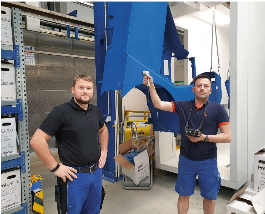
Benedikt Seidel, foreman and head of the painting technology department (left) in conversation with shift foreman Turo Zoltan (both from the Brückner Group), who checks the workpieces with the mobile measuring device – here a blue fuel tank for a feed mixer.
