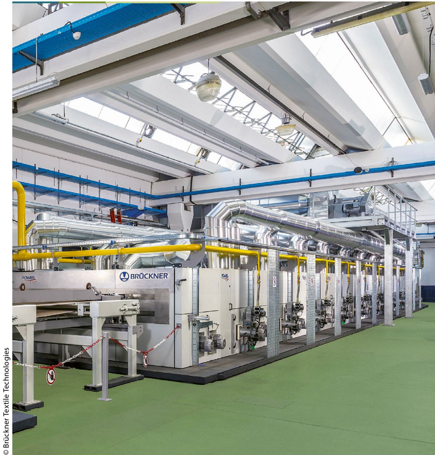
The stenter frame is the heart of textile finishing.
