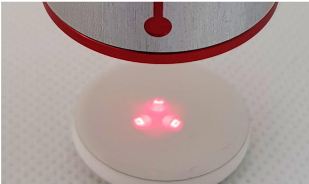
Figure 11: Incorrect distance to the measurement object
